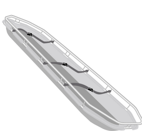
Image 3a: Mounting the patient restraint belts in the SAN-0087-1-M
