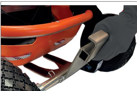
③ Attach the fully assembled base plate to the edge of the basket stretcher by flange-mounting the base plate bracket to the edge of the basket stretcher. Please always use the foot side of the basket stretcher.
