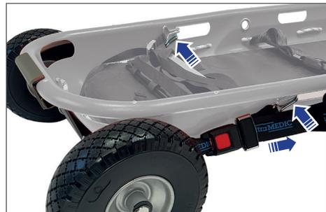
④ Hook the straps into the recessed grips and tighten.
